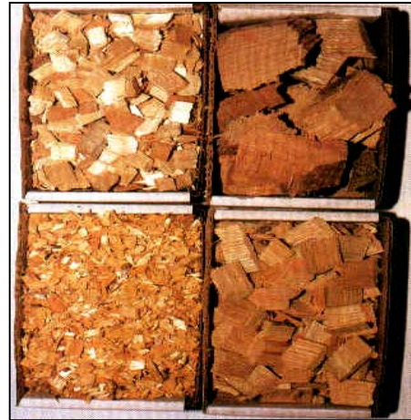
Figure 7.1: For some machines, chip size can be regulated between \frac{1}{4} and 1 inch landscape chips.
